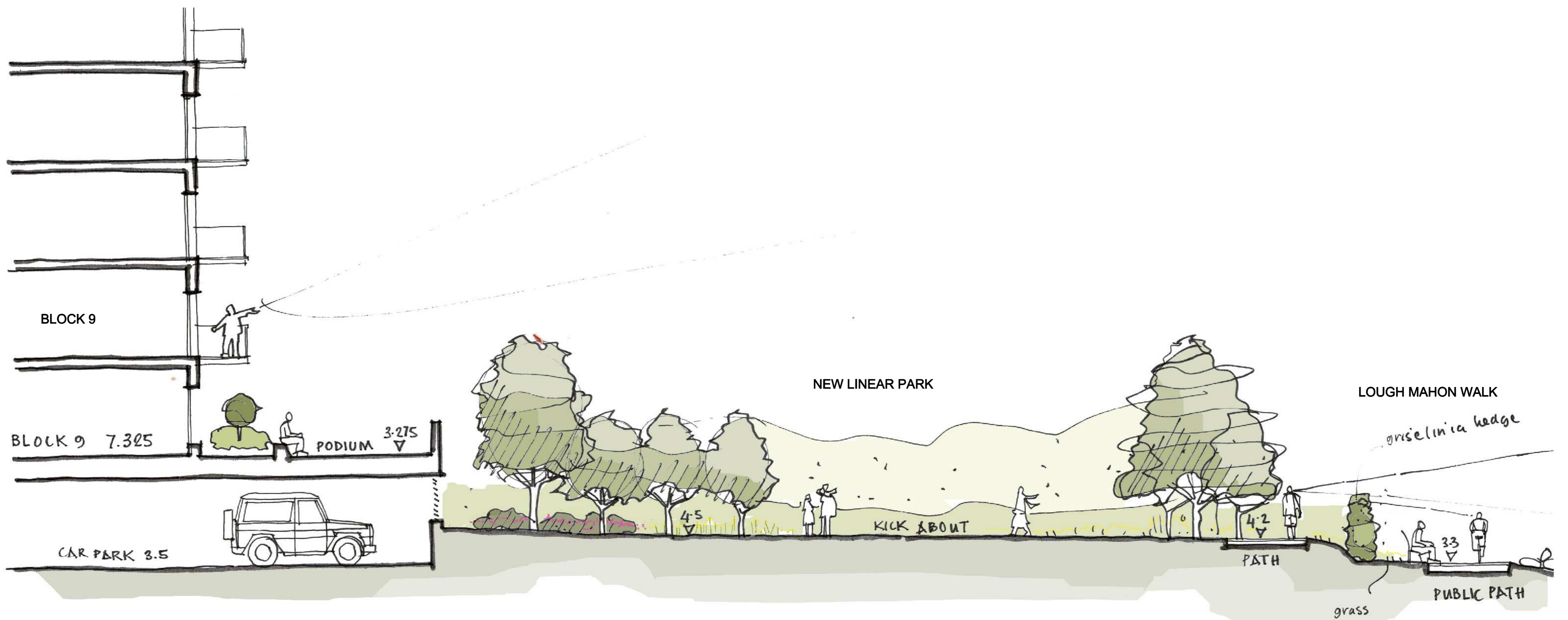
Section through Block 9 and the Interface with Mahon Walk illustrating the relationship between the apartments, podium deck over car park, linear park and Lough Mahon Walk
