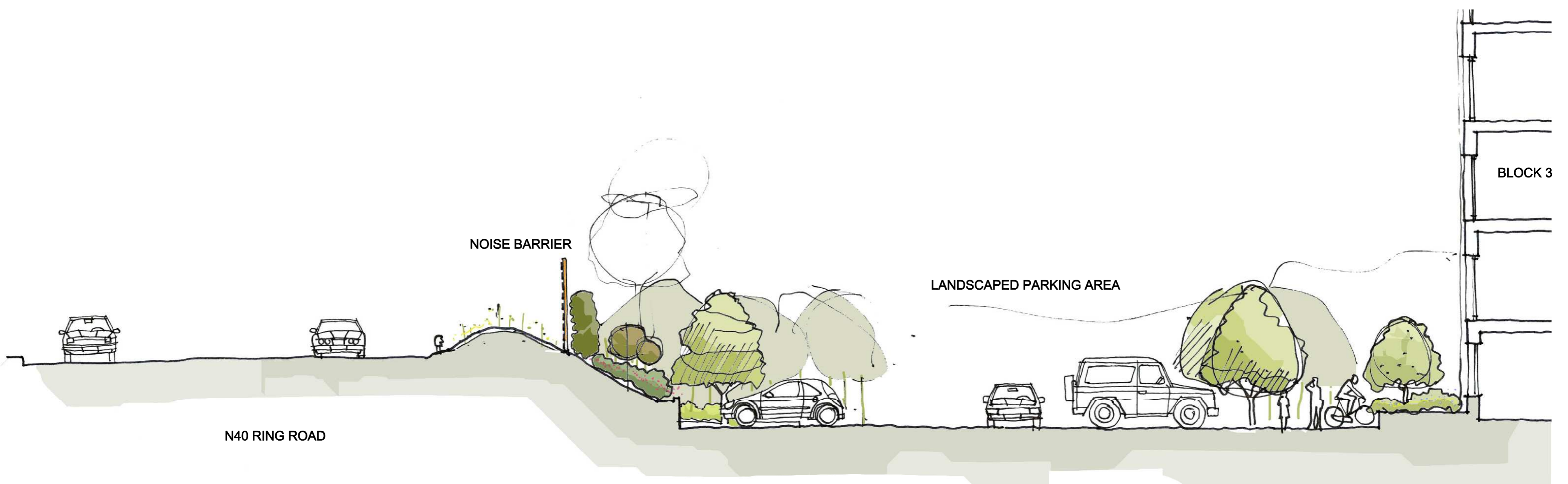
Section through Block 3 and the Interface with the N40 Ring Road illustrating the relationship between the apartments, noise barrier and the ring road
